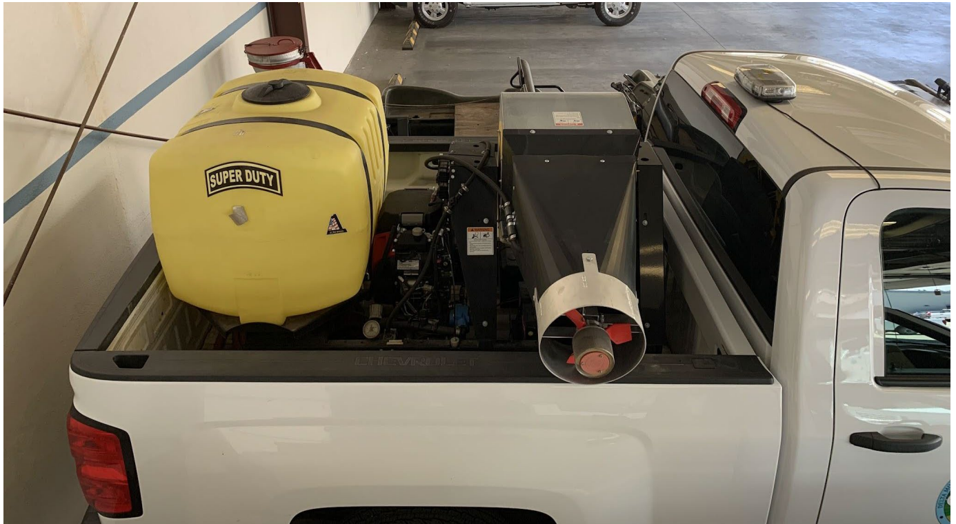
Figure 2. Example of a Wide Area Larviciding System mounted on a truck.
