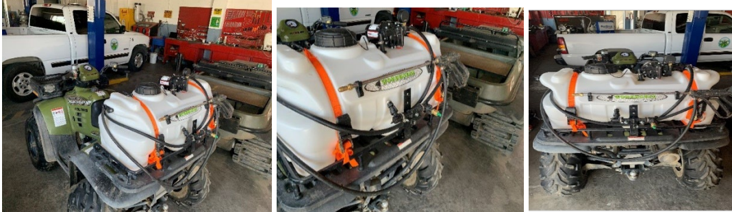
Figure 2. Photos showing the boomless spray mounted on the Quad four-wheeler all-terrain vehicle.
