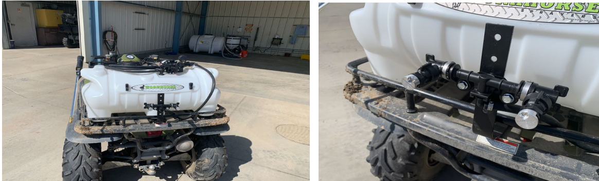
Figure 5. A photo showing the upgraded Quad with a new pesticide tank and boomless spray.
