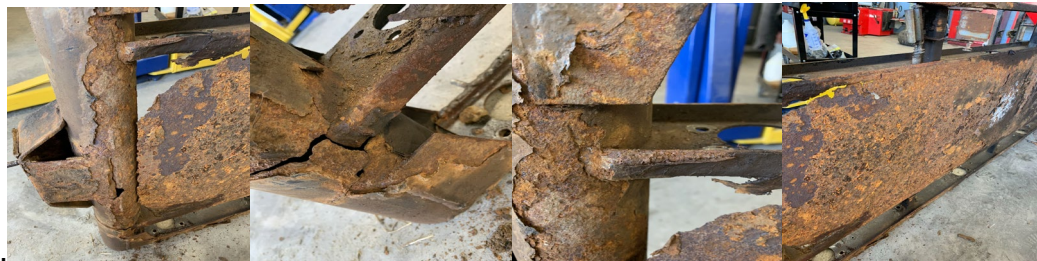
Figure 3. Image of extensive damage to T-29 Argo from rust and cracks.
