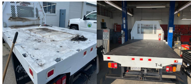
Figure 2. Image of the before and after restoration of Truck (T-4) flatbed.
