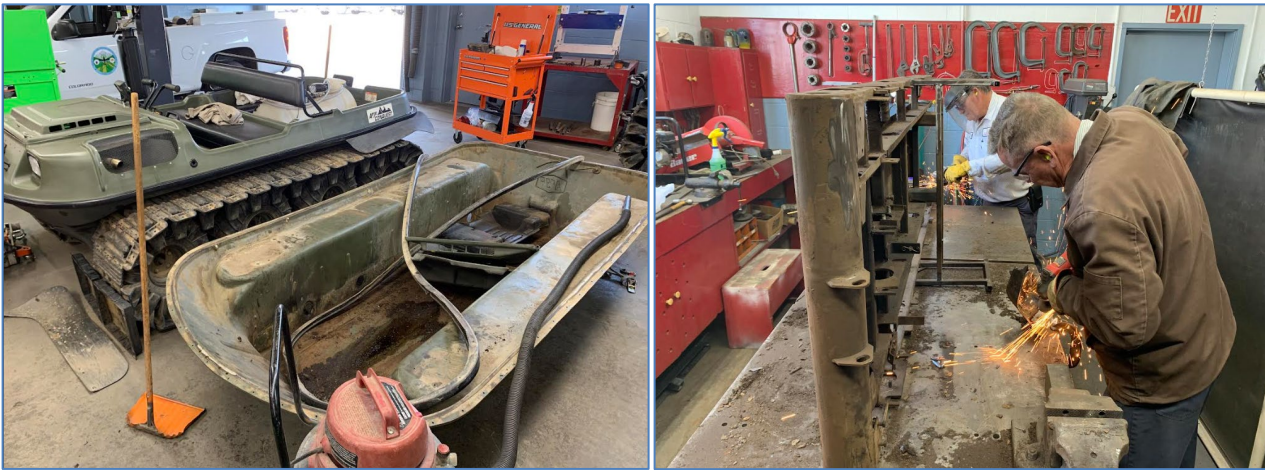
Figure 3. Image comparison of an ARGO and an ARGO tear down. Paul Harlien and Paul Raper refurbishing T-29 ARGO frame.
