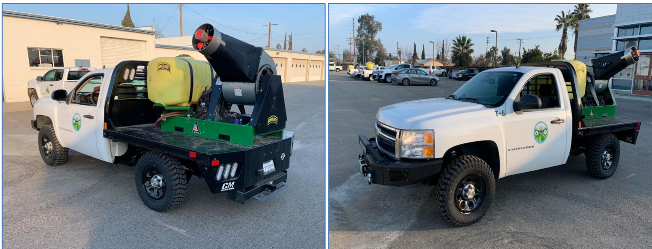
Figure 2. Vehicle T-6 post update photo of the flatbed, front bumper, winch, and A-1 Super Duty installation.
